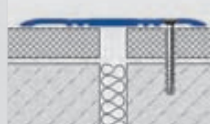
DURAFLEX series KA Aluminium/stainless steel Smooth or ribbed surface held with screws on one side
